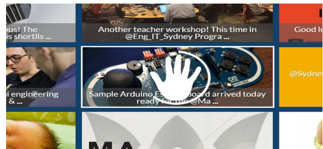
Figure 4. Hand icon representing the cursor, which is mapped to the user’s hand movement, and the loading circle providing visual feedback when hovering selectable items.
